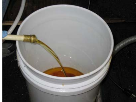
Figure 5. Draining biodiesel layer.
